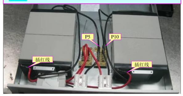
$2_{\times}$  As below shown, lock the baffle of battery on the base. Screw: 38-000008 - XXG \* 4; Torque: 8 KGF - CM
